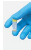
3. Plunge: Press the plunger slowly over ~three seconds to filter the sample
