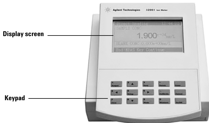
Figure 6 The front view of the 3200I Ion Meter
