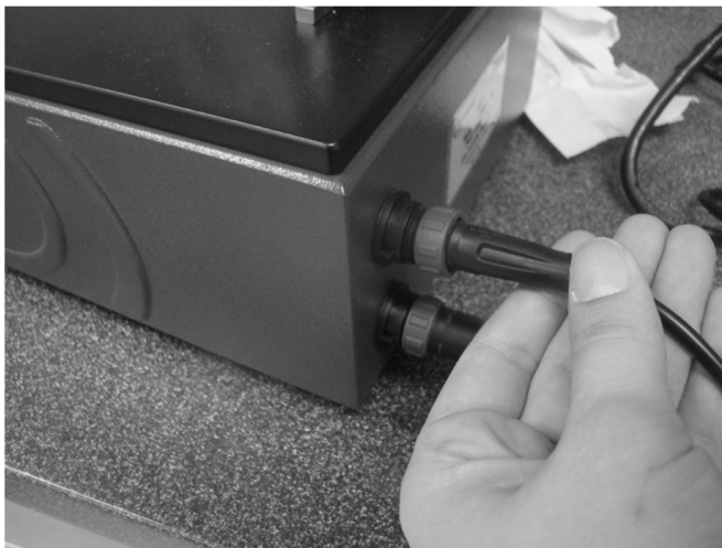
Figure 3. Attaching the USB cable
