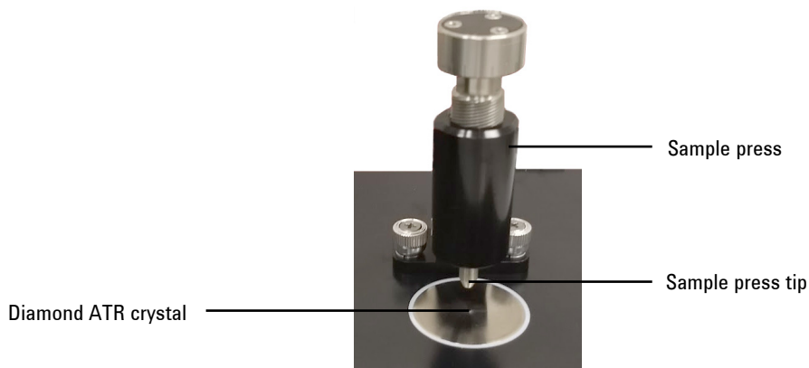
Figure 7. Sample press in highest position providing easy access for sample loading and cleaning
