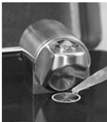
Figure 6. Applying a sample to the bottom window on the Tumbler
