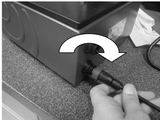
Figure 1. Attaching the power cord
