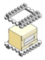
8 Slide the instrument into the outer cardboard box.
