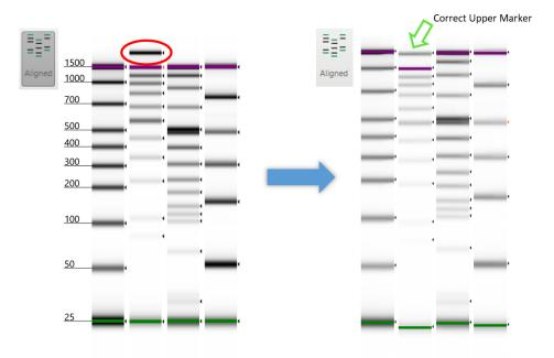
Figure 26 Example of an incorrect (Left) assigned Upper Marker and how to identify the correct Upper Marker (Right) in the D1000 ScreenTape assay in the TapeStation Analysis software.
