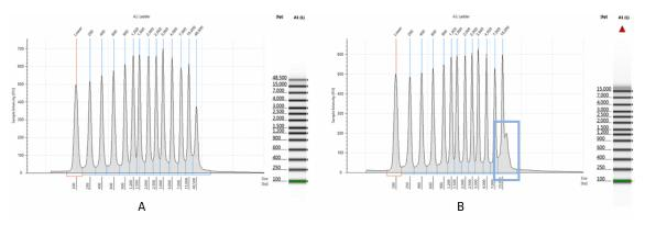
Figure 43 The effect of vigorous shaking of the Genomic DNA Ladder. A) Genomic DNA Ladder has been handled as directed prior to analysis on the Genomic DNA ScreenTape assay. B) The Genomic DNA Ladder vial was handled incorrectly - degradation of the top fragment (48500 bp) is clearly shown.
