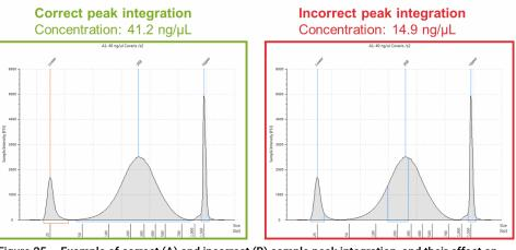
Figure 25 Example of correct (A) and incorrect (B) sample peak integration, and their effect on reported sample concentration.
