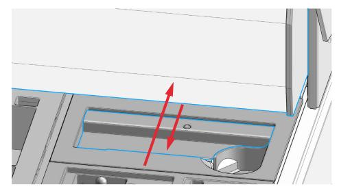
The lower nest cover mounting is correct if it moves smoothly in opposite direction to the gantry cover.
