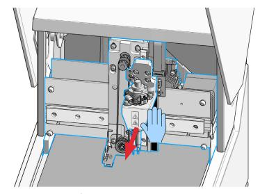
**3** Place lower slot opening of the gantry cover onto the lower peg with conical head (30°).
