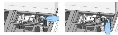
**2** Mount the lower nest cover to the lever such that the half-round cutout meets its counter part on the lever.
