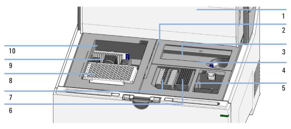
1 Gantry cover 2 Upper nest cover 3 Lower nest cover 4 ScreenTape nest 5 Tip waste 6 Tip rack 7 Tube strip holder 96-well sample plate 8 9 ScreenTape rack 10 ScreenTape waste location
