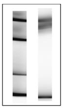
Figure 15 Effect of bubbles at the gel interface on TapeStation Analysis software results - Gel view/unaligned
