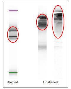
Figure 16 Different effects of bubbles in the gel matrix on TapeStation Analysis software results - Gel view
