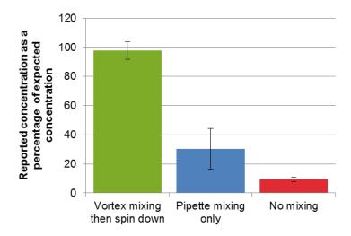
Figure 20 Chart of reported concentrations for the ScreenTape reagent mixing tests, using the D1000 ScreenTape assay.
