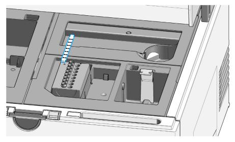
**16** Ladder is exclusively provided from location A1 on the sample tube strip holder. For further details on handling the ladder within assays see the assay-specific Quick Guides or the section "Ladder Considerations" on page 98.
