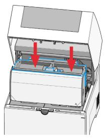
**12** Push the gantry carefully towards the back of the instrument.
