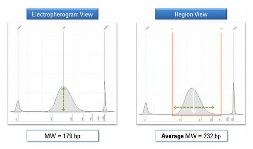
Figure 27 The sizing data obtained in Electropherogram and Region views of the TapeStation Analysis software.
