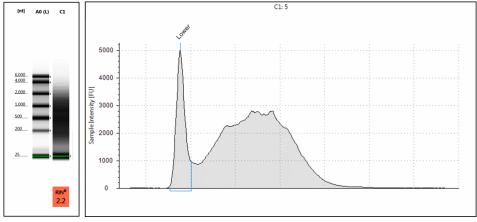
Figure 23 Example of a degraded RNA sample in the High Sensitivity RNA assay resulting in missing peak identification in the Gel View (Left) and Electropherogram View (Right) of the TapeStation Analysis software.
