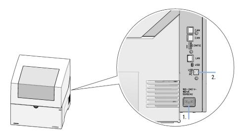
1. Power line in, 2. USB-B to PC Remaining connectors are blocked by plugs and reserved for factory use.
