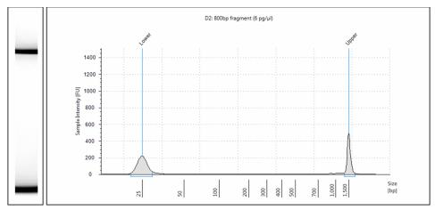
Figure 32 Example of missing sample peak due to too low concentrated sample in the High Sensitivity D1000 assay in the Gel view (Left) and Electropherogram view (Right) of the TapeStation Analysis software.
