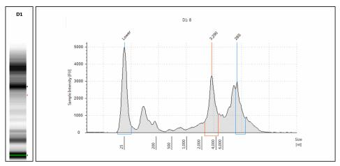
Figure 22 Example of extra peaks being detected at the 28S position due to insufficient denaturation in the Gel View (Left) and Electropherogram View (Right) of the TapeStation Analysis software.
