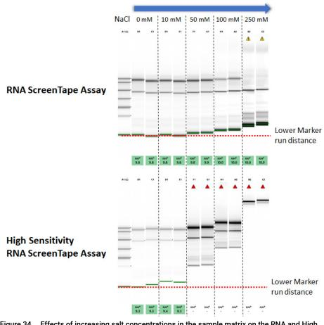
Figure 34 Effects of increasing salt concentrations in the sample matrix on the RNA and High Sensitivity RNA Screentape Assay in the unaligned Gel view of the TapeStation Analysis software. **RINe Functional Range**
