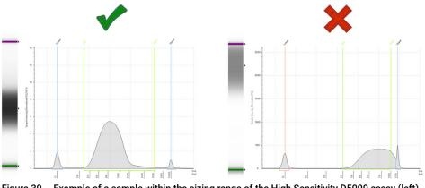
Figure 30 Example of a sample within the sizing range of the High Sensitivity D5000 assay (left) and the same sample merging with the upper marker (right) in the High Sensitivity D1000 assay.
