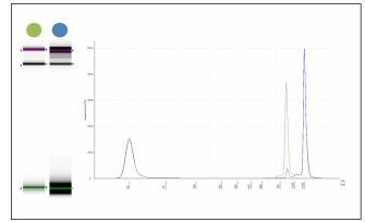
Figure 44 Example of intense upper and lower markers seen in the blue gel image. Lower markers are normalized in electropherogram view and appear identical in signal.
