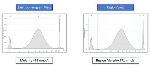
Figure 28 The concentration data obtained in Electropherogram and Region views of the TapeStation Analysis software.
