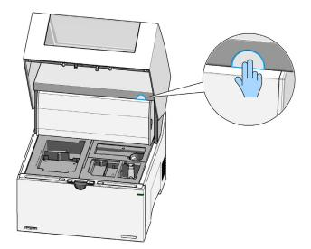
Pressing the release button of the transportation lock frees parts of the robotics from internal clamping. This mechanical unlocking activity enables the robotics to move and the instrument to operate. See details on transportation lock ("Transportation Lock G2991A" on page 167).
