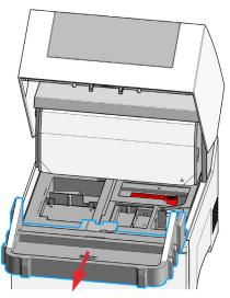
2 Carefully pull the gantry towards the front of the instrument.
