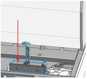
**17** Move the lever to the lock position.
