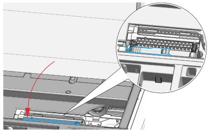
An internal locking bolt positions the Electrode Cartridge correctly.
