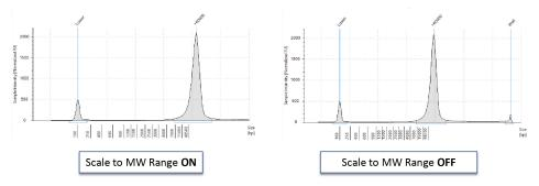
Figure 42 Visualizing a well peak in the Electropherogram view of the TapeStation Analysis software.
