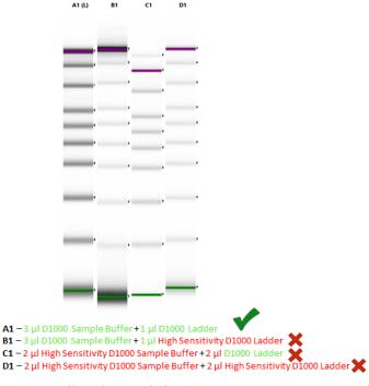
Figure 17 Effect of correct (A1) and incorrect consumables/protocol (B1 – D1) on the D1000 Ladder peak intensity and Marker assignment in the D1000 ScreenTape assay.
