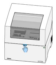
4 Insert a TapeStation Test Tape.
