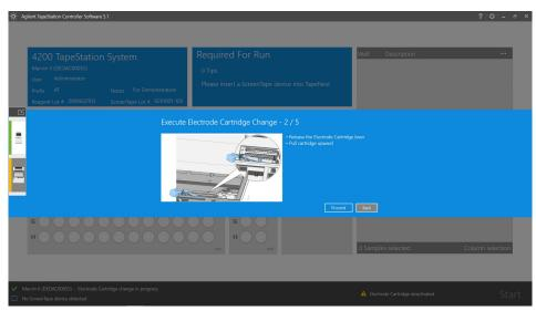
**13** Release the cartridge lever with a push and bring it to the upright position.
