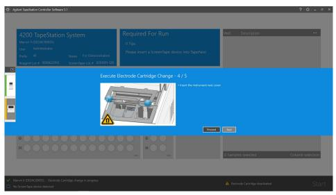
**19** Reinsert the upper nest cover: Guide the rear positioning extensions into the corresponding recesses under the gantry. Lower the cover until the magnets hold it in place.
