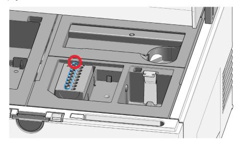
**17** Alternatively, samples can be run from a sealed 96-well sample plate by inserting a sealed 96-well sample plate in correct orientation (The letters A to H are embossed for reference on the left hand side of the recess for the 96-well sample plate). Vortex and centrifuge 96-well sample plates before insertion.
