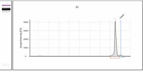
Figure 31 Example of missing marker peak due to too concentrated sample in the High Sensitivity D1000 assay in the Gel view (Left) and Electropherogram view (Right) of the TapeStation Analysis software.
