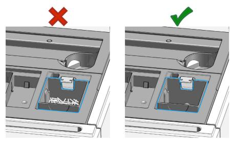
4 Remove the sample tube strip.
