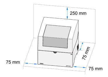
Allow approximately 75 mm (3 inches) of clear space around the instrument for air circulation and electrical connections.
