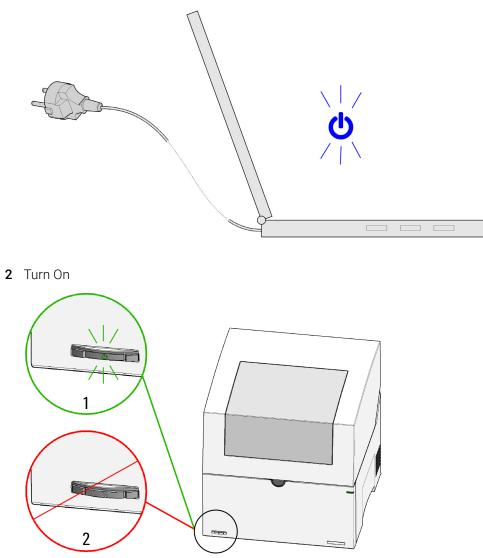
Figure 14 Power switch. 1: On; 2: Off
