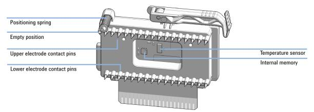
Figure 40 Electrode Cartridge front view for the 4200 TapeStation system (G2991B) and 4150 TapeStation system (G2992A)
