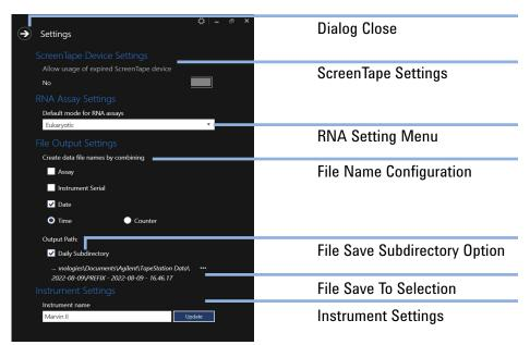
Figure 10 TapeStation Controller software settings dialog box
