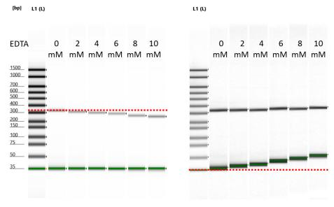
Figure 45 Effect of increasing EDTA concentration on lower marker run distance in aligned (left) and unaligned (right) gel view in the TapeStation Analysis software.
