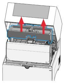
4 Push the gantry carefully towards the back of the instrument.
