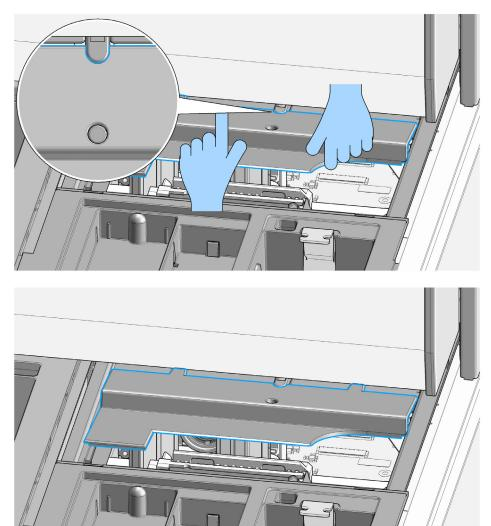
**3** Reinsert the upper nest cover: Guide the rear positioning extensions into the corresponding recesses under the gantry. Lower the cover until the magnets hold it in place.
