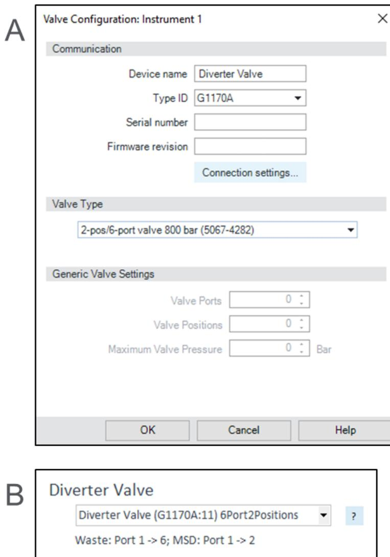
**Figure 3** Configuration of the diverter valve in the ChemStation Instrument Configuration (A) and the 2D-LC Configuration (B).
