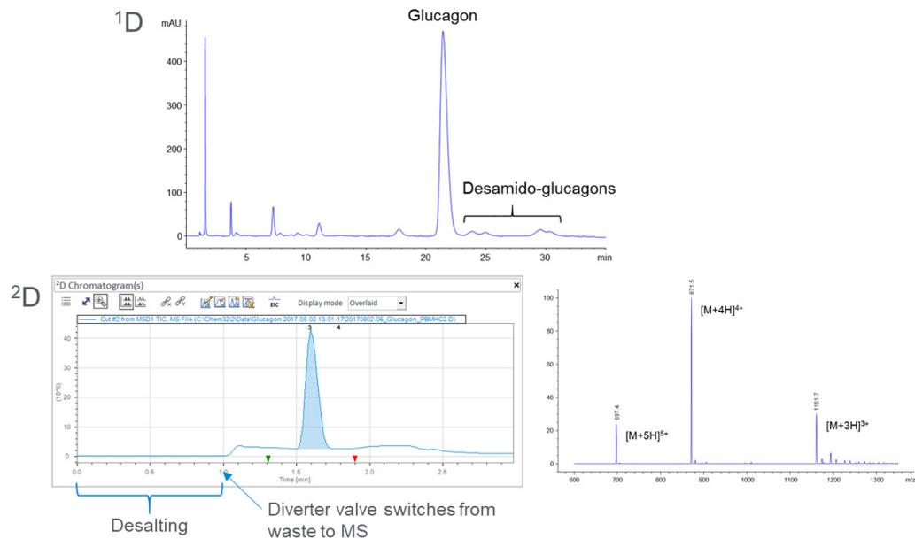
**Figure 1** Peak-based multiple heart-cutting 2D-LC analysis of the peptide glucagon.
