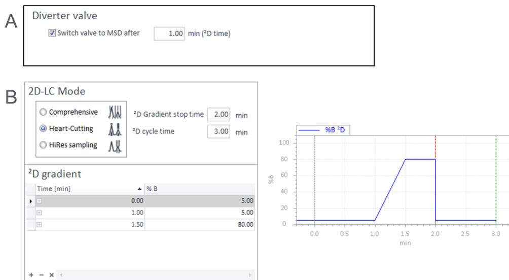
**Figure 4** 2D-LC method setup for diverting salt or buffers originating from the <sup>1</sup>D mobile phase to waste at the beginning of every <sup>2</sup>D run, (A) diverter valve setup in the **Advanced settings** tab of the 2D-LC method, (B) <sup>2</sup>D gradient setup in the **General settings** tab of the 2D-LC method.
