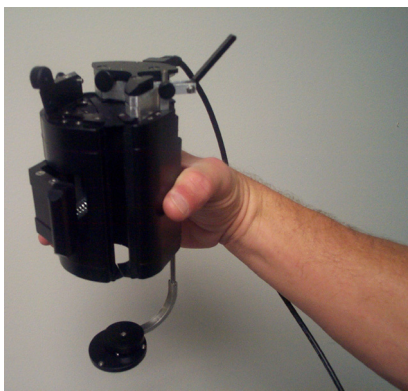
Figure 28. Proper Hand Position to Zero Diameter Arm
