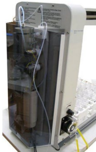
Figure 21. Agilent SPS 3 autosampler with optional Diluter installed
