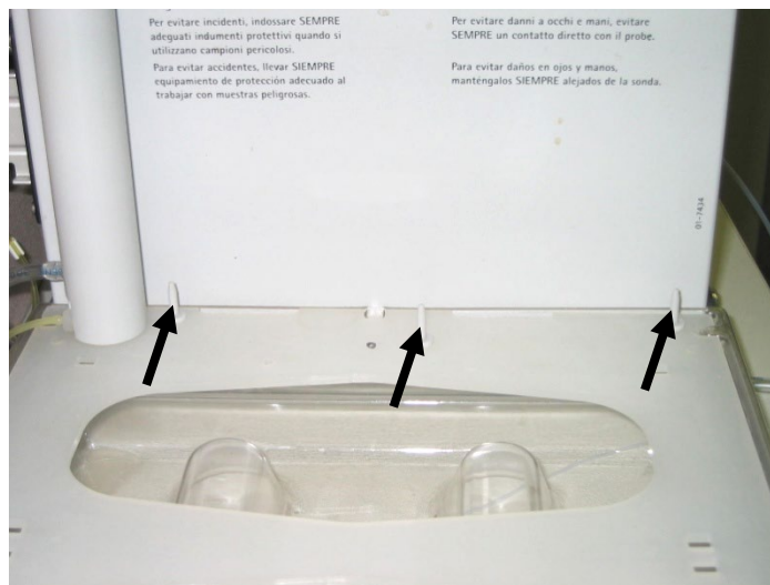
Figure 11. Standards rack locating pins correctly installed
