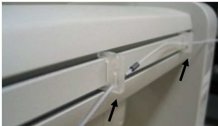
Figure 16. Location of tube-retaining clips
