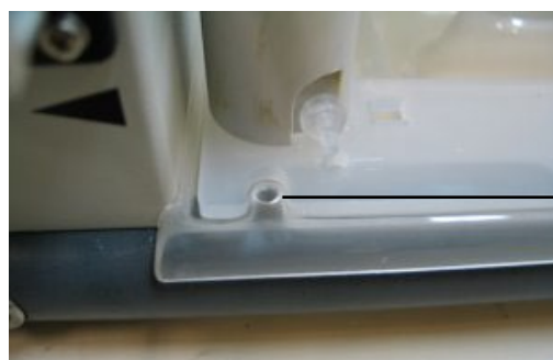
Figure 3. The locating alignment pin on the spill tray
