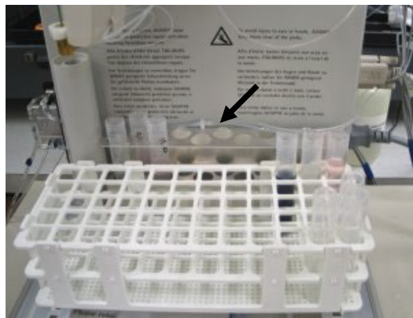
Figure 13. Standards rack installed on Agilent SPS 3
