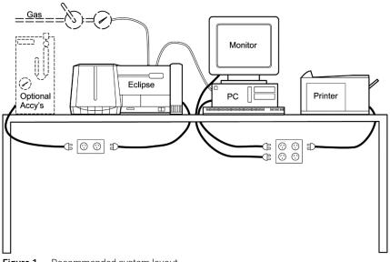
Figure 1. Recommended system layout
