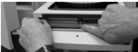
Figure 17 Replacing the syringe block assembly and syringe
