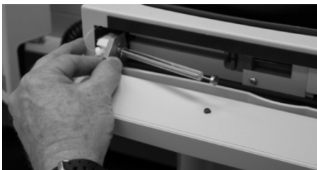
Figure 16 Removing the syringe block assembly and syringe
