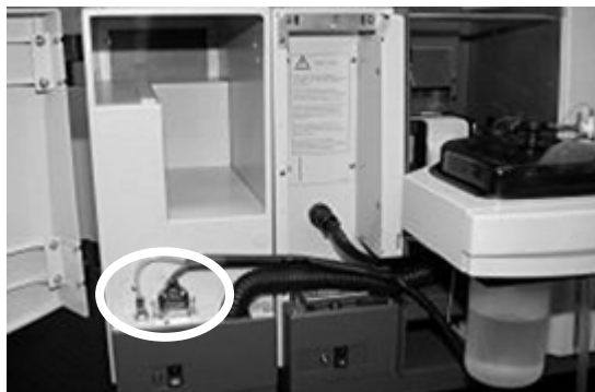
Figure 7 Location of the PSD gas and control cable connectors on the GTA
