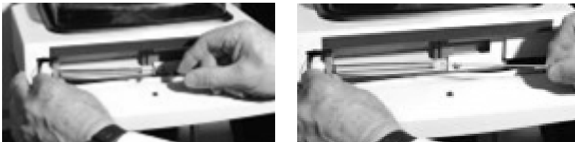
Figure 18 Removing the plunger of the syringe
