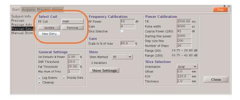
Figure 8. Selecting a Coil on Prescan Setup Page
