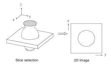
Figure 54. 2D Image Resulting from a Slice Selection
