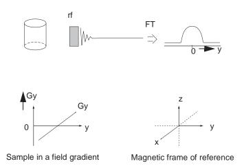
Figure 52. Effect of a Field Gradient Along Direction y
