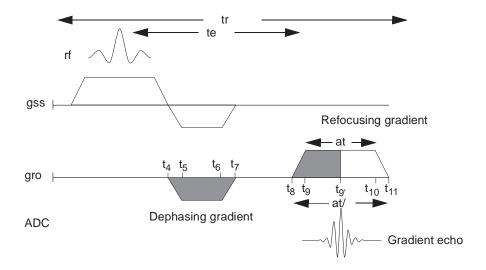
Figure 60. Readout Gradient and Gradient Echo
