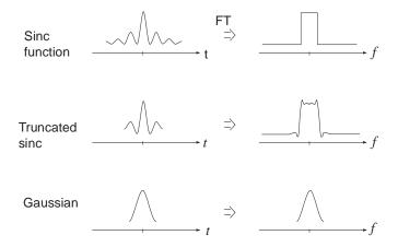
Figure 57. Sinc Function, Truncated Sinc Pulse, and Gaussian-Shaped Slice Profiles
