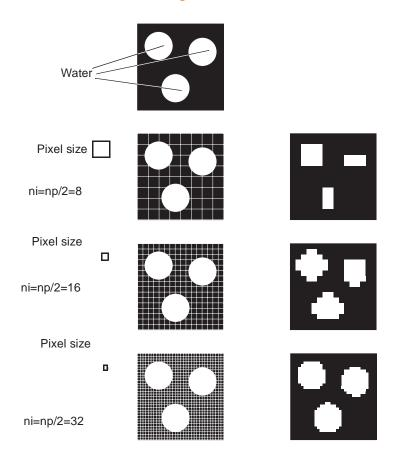
Figure 62. Image Resolution of Three Water-Filled Spheres
