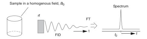
Figure 51. Frequency Spectrum Produced by an NMR Signal
