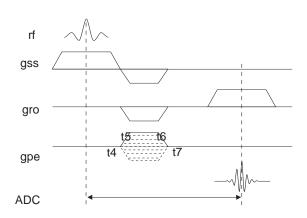
Figure 61. Gradient Echo Imaging Sequence
