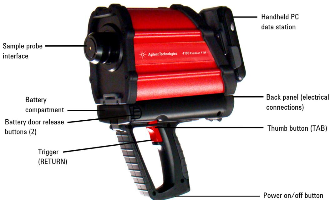
**Figure 1.** Agilent 4100 ExoScan FTIR
