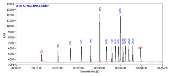
Representative NGS DNA Ladder result using the Fragment Analyzer systems with the DNF-473 NGS Fragment kit (1–6000bp). The peaks are annotated by size (bp). Method: DNF-473-33 (short capillary array).
