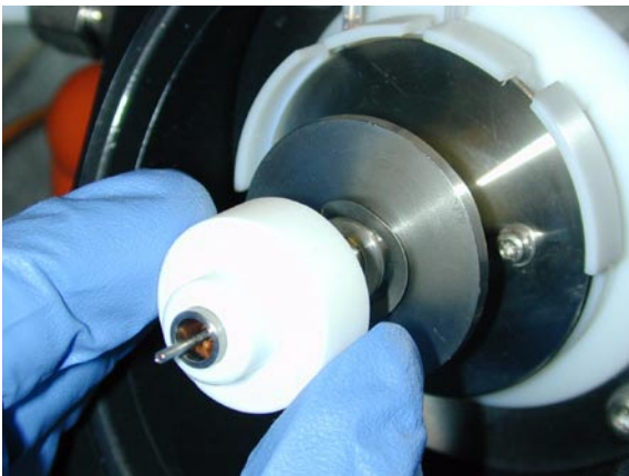
Figure 33 Slide the PTFE Centering Bushing over the Wave Disk Spring to finish the Capillary Extension Assembly
