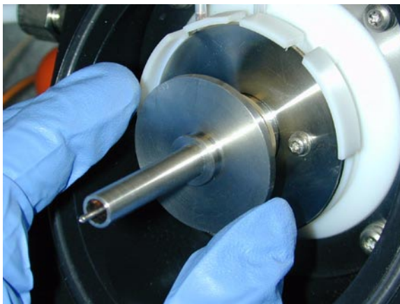
Figure 31 Install the Heating Sleeve over the Capillary Extension
