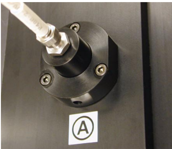
Figure 159 Loosen three setscrews to adjust fiber cable connector
