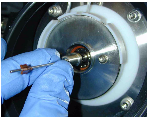
Figure 110 Install the Capillary Extension to the LC/MSD TOF
