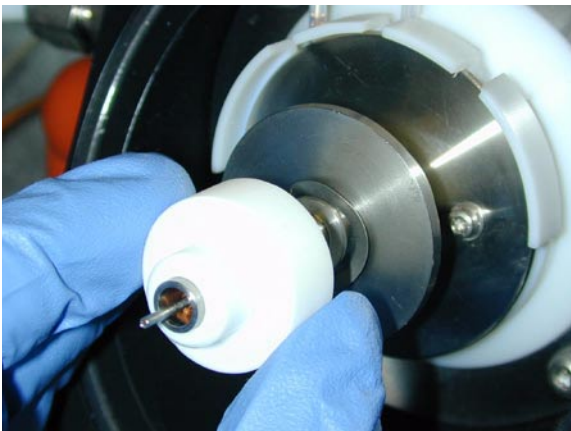
Figure 113 Slide the PTFE Centering Bushing over the Wave Disk Spring to finish the Capillary Extension Assembly
