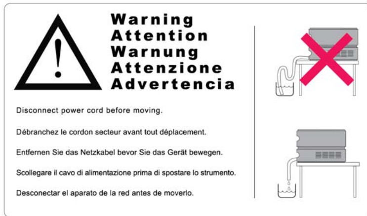
Figure 13 Warning label (illustration for correct waste tubing)
