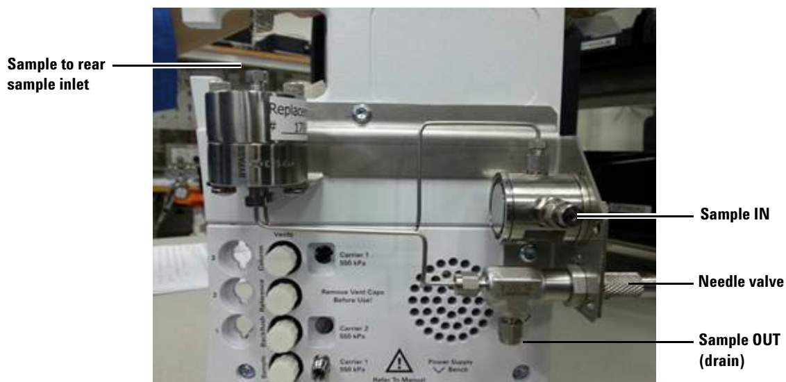
Figure 22 G3581-S0003 pressure regulator assembly installed
