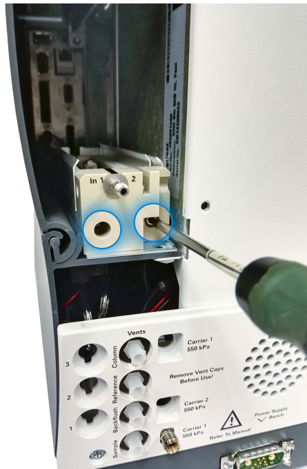
Figure 16 Remove the PEEK block by unscrewing two bolts.
