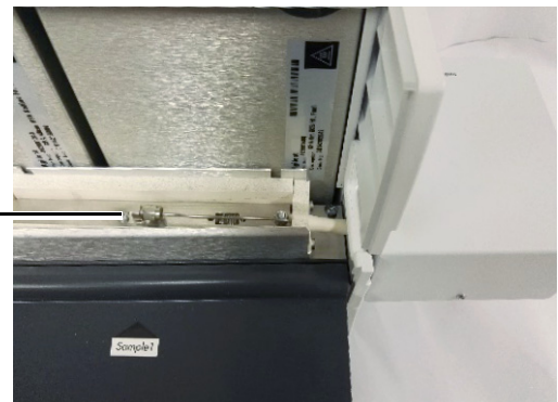
Figure 17 Install the back panel and micro-gasifier, and connect the micro-gasifier sample line to the internal sample inlet using a 1/16-inch Swagelok fitting.
