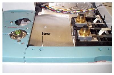
Figure 5 Install valve box blanking plate
