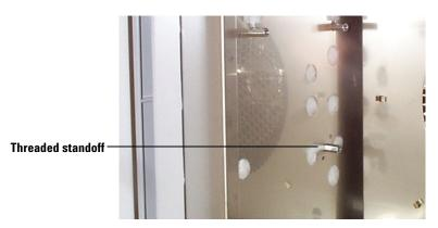
Figure 18 Standoff in screw mount
