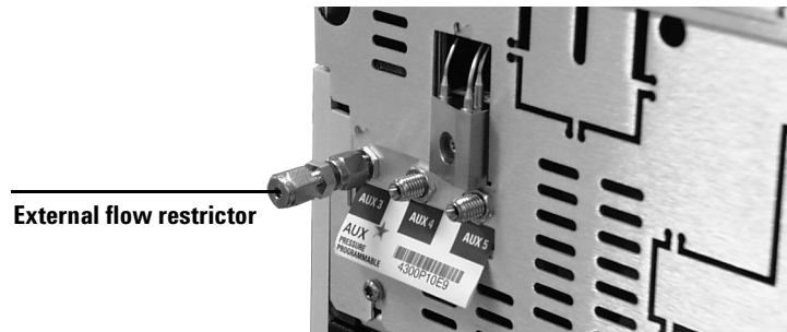
Figure 3 External flow restrictor installed and ready for connection to gas line
