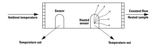
Figure 5 Measuring the leak rate
