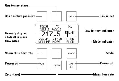
Figure 2 Flow mode screen/buttons
