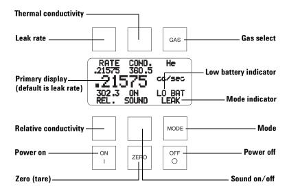
Figure 4 Leak detector mode screen/buttons
