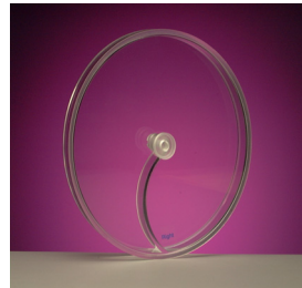
Figure 2 Traditional Roche-type USP drum with a single-chamber design
