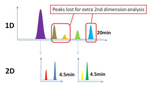
This problem is addressed using a setup called *multiple heart-cutting* 2D-LC. Here, the sampling loops on the 2D-LC valve are exchanged with 6-position/14-port selection valves, which are equipped with six loops each. In this configuration, a peak can be cut out and stored, then analyzed as soon as the second dimension is free.
