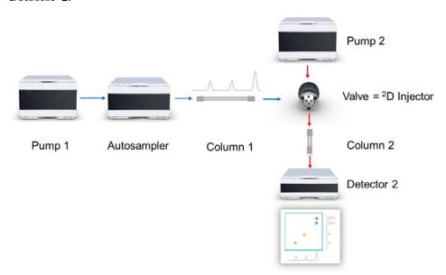
Figure 1 Concept of a 2D-LC-System
