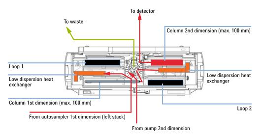
Figure 9 Columns at different temperatures, medium 1<sup>st</sup> dimension column, no 1<sup>st</sup> dimension detector
