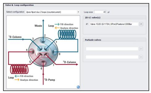
Figure 23 2D-LC valve and loop configuration
