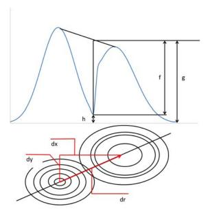
Figure 109 Diagram of 2D resolution measurement: Slice for resolution (top) and 2-dimensional contour plot (bottom)
