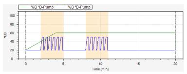
In the upper case, the second dimension solvent gradient does not change, despite the changing composition of the solvent in the first dimension.
