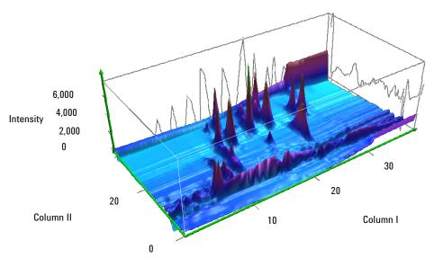
Figure 106 3-Dimensional display of the separation of the 26 compound standard mixture. The first dimension separation takes 40 minutes and each second dimension separation takes 39 seconds. The back side shows a generated first dimension chromatogram and gives the impression which peaks are coeluting and separated in the second dimensions.
