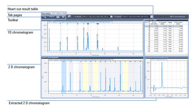
Figure 39 Overview of the 2D-LC Heart-Cut Viewer graphical user interface
