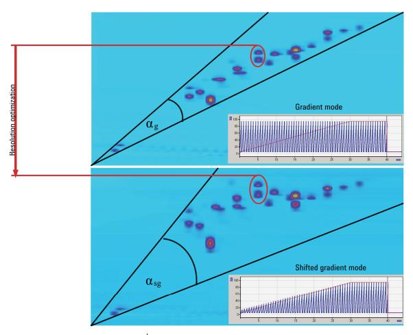
Figure 118 2<sup>nd</sup> dimension gradient mode compared to isocratic mode and its effect on resolution
