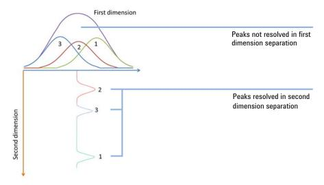
Figure 107 Peak capacity relationship between peak capacities of orthogonal first and second dimension
