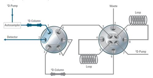
Figure 86 Setup for 1D-LC analysis
