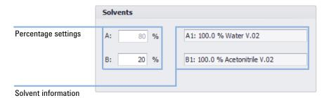
Figure 64 2D-LC solvent settings
