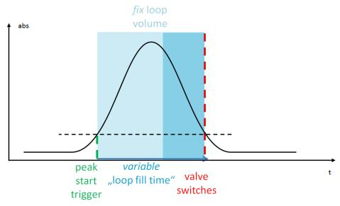
Figure 6 Peak triggering concept (signal falls below threshold or slope)
