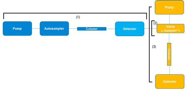
Figure 112 Diagram of instrumentation for 2D-LC
