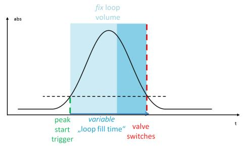
Figure 47 Peak triggering concept (signal falls below threshold or slope)
