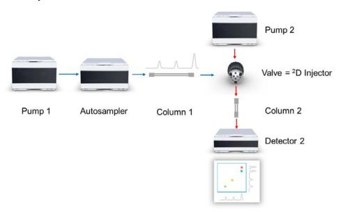
Figure 81 Concept of a 2D-LC-System
