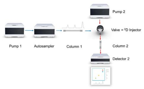
Figure 123 Concept of a 2D-LC-System
