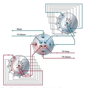
Figure 52 Valve setup with two 6/14 valves for peak parking
