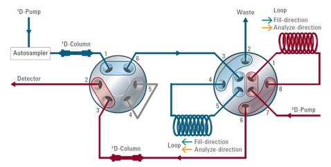
Figure 54 Setup for 2D-LC analysis
