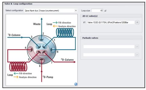
Figure 94 2D-LC valve and loop configuration
