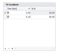
The time axis relates to the Stoptime of the  $2^{nd}$  dimension pump. **Time** [min] = 0.00 marks the start of the maybe repetitive gradient cycles, a time greater than **Stoptime 2D** will be ignored.
