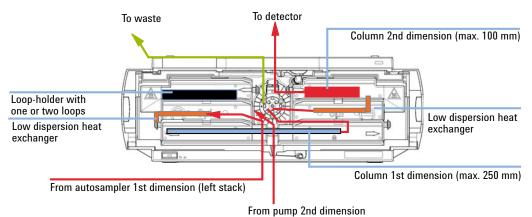
Figure 121 Columns at different temperatures,long 1<sup>st</sup> dimension column, no 1<sup>st</sup> dimension detector, for comprehensive 2D-LC booth loops can be placed in the loop holder.
