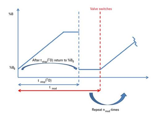
Figure 74 Characteristics of LCxLC
