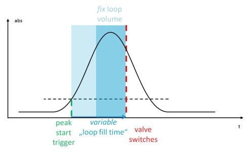
Figure 46 Peak triggering concept (elapsed sampling time)
