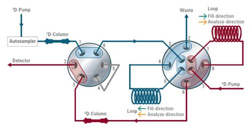
Figure 87 Setup for 2D-LC analysis
