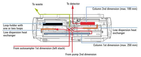
Figure 79 Columns at different temperatures,long 1<sup>st</sup> dimension column, no 1<sup>st</sup> dimension detector, for comprehensive 2D-LC booth loops can be placed in the loop holder.
