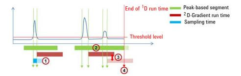
Figure 25 Heart cutting 2D-LC (general considerations) (delay times have been omitted for clarity, besides threshold also the peak-slope can be used for peak detection)
