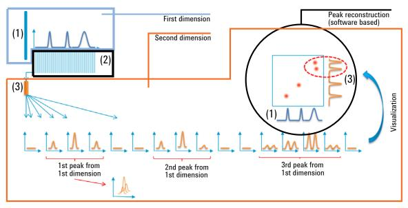
Figure 113 Principle of 2D-LC (example for LCxLC): Effluent of first column (1) is sampled (2) and injected to second column (3). Peaks of second column separation are detected and reconstructed.
