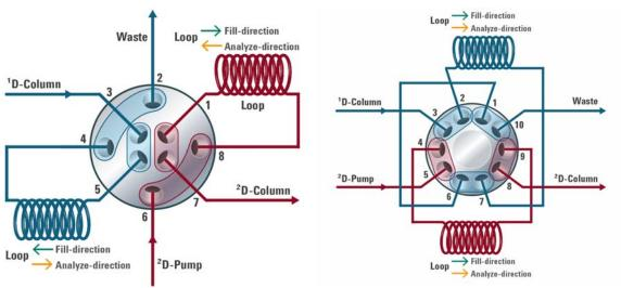
Figure 26 Valve and loop setup for heart-cutting 2D-LC with the 2D-LC Valve (dual-loop setup)
