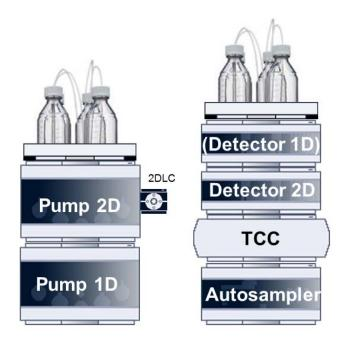
Figure 78 Stack configuration for Standard Heart-cutting 2D-LC
