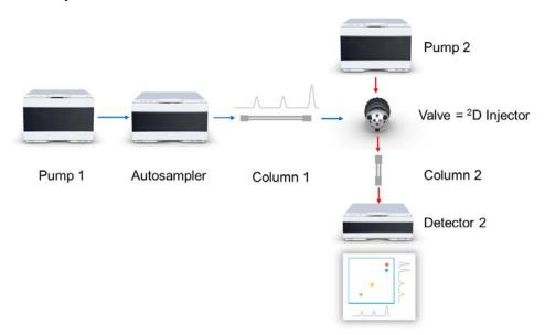
Figure 10 Concept of a 2D-LC-System
