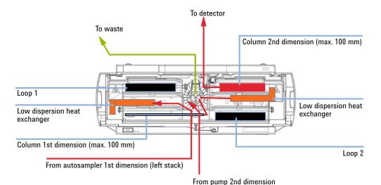
Figure 122 Columns at different temperatures, medium 1<sup>st</sup> dimension column, no 1<sup>st</sup> dimension detector
