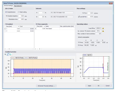
Figure 114 Standard gradient mode
