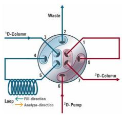
Figure 31 Valve and loop setup for heart-cutting 2D-LC with 2D-LC Valve
