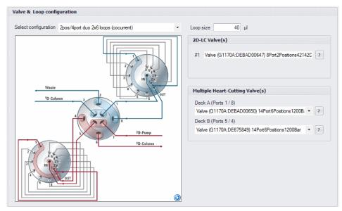
Figure 61 2D-LC valve and loop configuration
