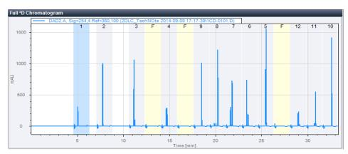
Figure 42 <sup>2</sup>D Chromatogram (example - only visible, if <sup>2</sup>D chromatogram (checkbox) is checked)
