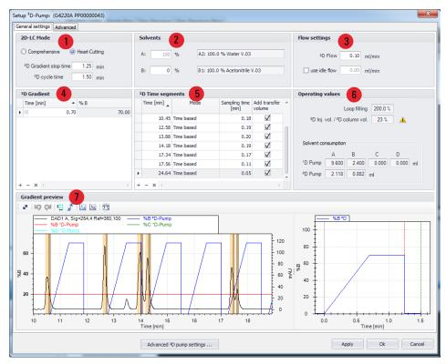
Figure 62 2D-LC method setup (General settings)
