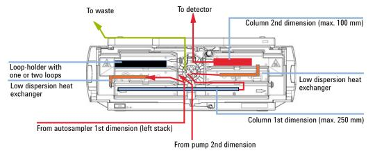
Figure 49 Columns at different temperatures,long 1<sup>st</sup> dimension column, no 1<sup>st</sup> dimension detector, for comprehensive 2D-LC booth loops can be placed in the loop holder.
