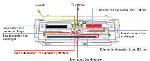
**Figure 8** Columns at different temperatures,long 1<sup>st</sup> dimension column, no 1<sup>st</sup> dimension detector, for comprehensive 2D-LC booth loops can be placed in the loop holder.
