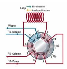
Figure 29 Valve and loop setup for heart-cutting 2D-LC with a 2/10 Valve (single-loop setup) - not recommended
