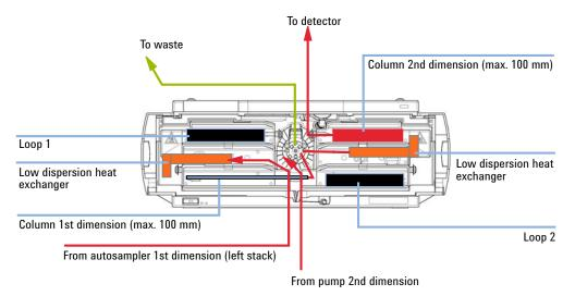
Figure 50 Columns at different temperatures, medium 1<sup>st</sup> dimension column, no 1<sup>st</sup> dimension detector
