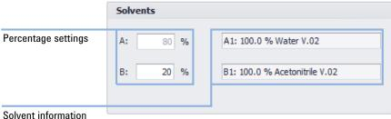
Figure 34 2D-LC solvent settings
