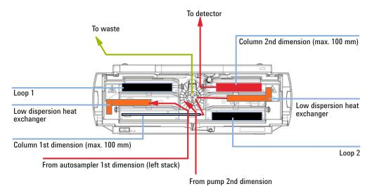
Figure 80 Columns at different temperatures, medium 1<sup>st</sup> dimension column, no 1<sup>st</sup> dimension detector
