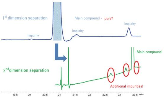
Figure 38 Example of a heartcutting 2D-LC experiment. Data analysis and display done by OpenLAB CDS ChemStation Edition, the data of a detector placed after the first dimension column (blue) and of the 2D data detector (green). The additional impurities (marked red) could not be detected by 1D-LC only.
