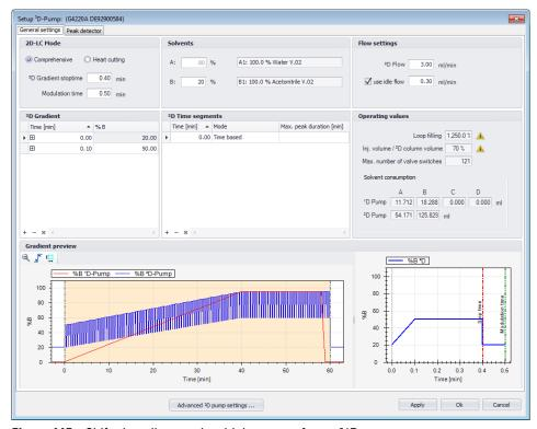
Figure 115 Shifted gradient mode with increase of start-%B
