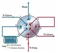
Figure 28 Valve and loop setup for heart-cutting 2D-LC with the 2D-LC Valve (single-loop setup)
