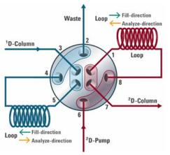
Figure 30 Valve and loop setup for heart-cutting 2D-LC with the 2D-LC Valve
