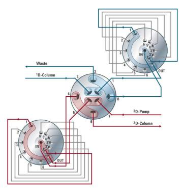
Figure 44 Valve setup with two 6/14 valves for peak parking
