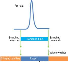
Loop connected to 1D-Column
