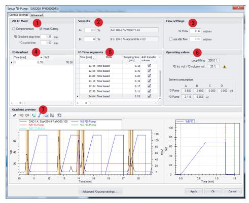
Figure 24 2D-LC method setup (General settings)
