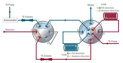
Figure 16 Setup for 2D-LC analysis
