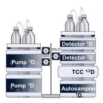
Figure 48 Stack configuration for Multiple Heart-cutting 2D-LC
