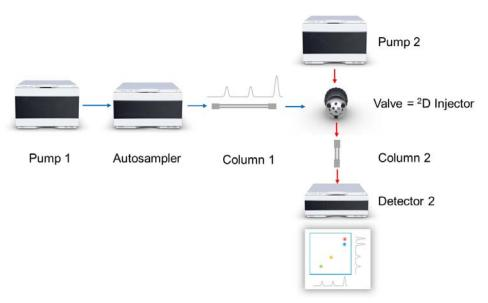
Figure 51 Concept of a 2D-LC-System
