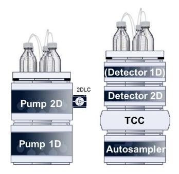
Figure 7 Stack configuration for Standard Heart-cutting 2D-LC
