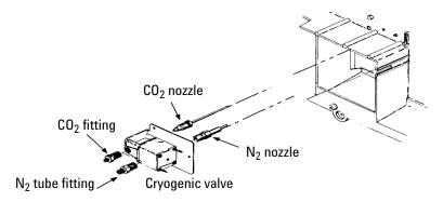
3. Route the two valve leads through the space between the oven and the mainframe, across the rear of the instrument, to the main circuit board.
