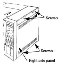
10. Remove the back cover of the instrument by removing four screws and sliding the cover off the rear of the instrument.
