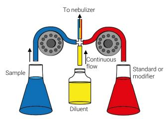
Figure 2 The SIPS 20 dual pump system
