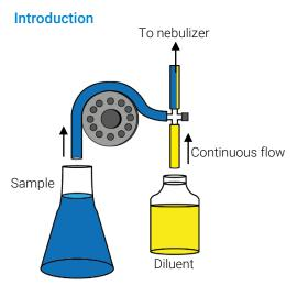
Figure 1 The SIPS 10 single pump unit
