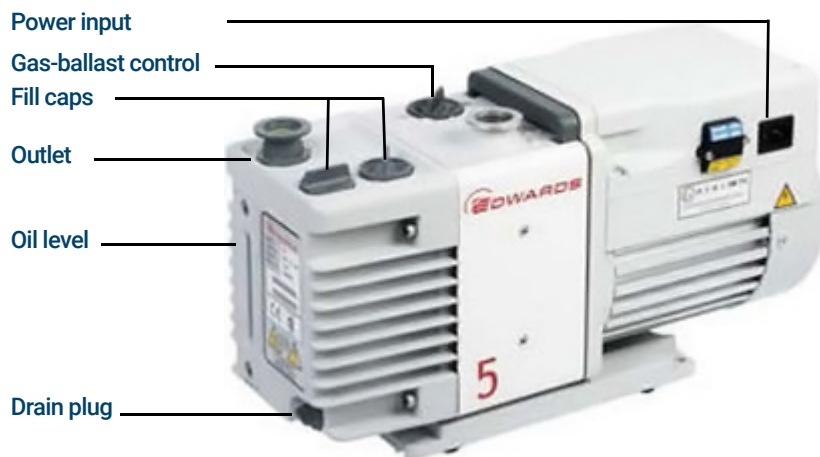
Figure 12. Rotary vane foreline pump
