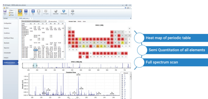
Figure 9. Intelliquant is a fast semi-quantitative data acquisition routine for ICP-OES that can collect data across the entire spectral range to provide quick sample insight.
