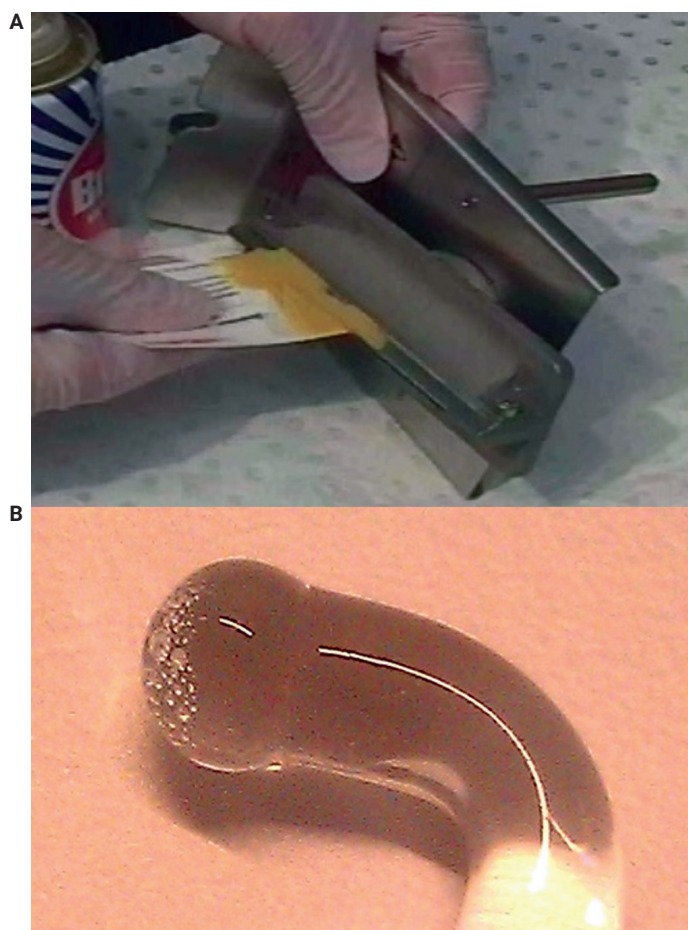
Figure 5. (A) Clean the burner by polishing using a metal cleaning fluid such as "Brasso" on the burner cleaning card. (B) The glass impact bead should be replaced if it is badly pitted.
