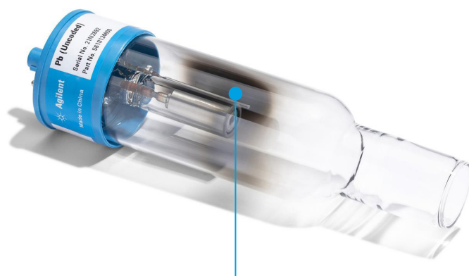
Figure 1. Characteristic black "getter" patch from unique lamp processing. May also see some cathode material deposited during lamp processing.
