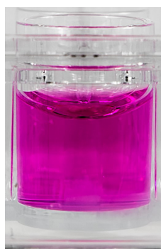
Figure 1. Microplate well demonstrating liquid meniscus effect.
