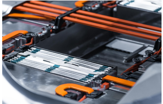
Figure 11. Internal section of electric vehicle battery pack with current connectors.
