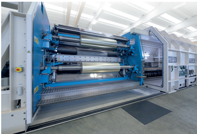
Figure 7. Interior section of a Roll-to-Roll vacuum deposition device.
