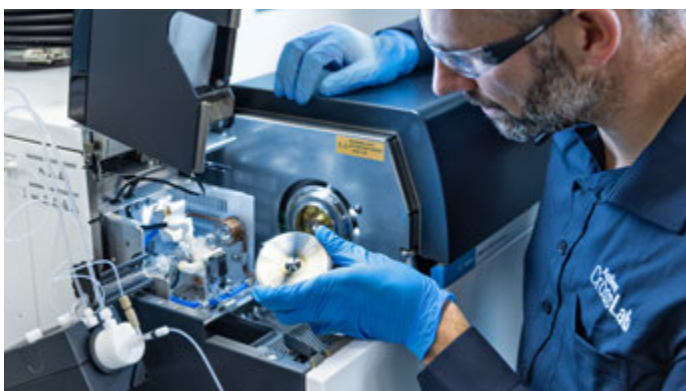
Figure 7. Visually inspect the cones.
