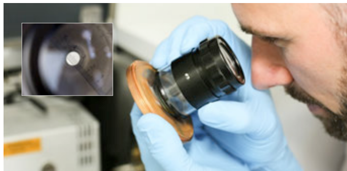
Figure 8. Agilent's LED measuring magnifier ( 5190-9614 ) is a tool to help users achieve optimum ICP-MS instrument performance and maximum cone life.
