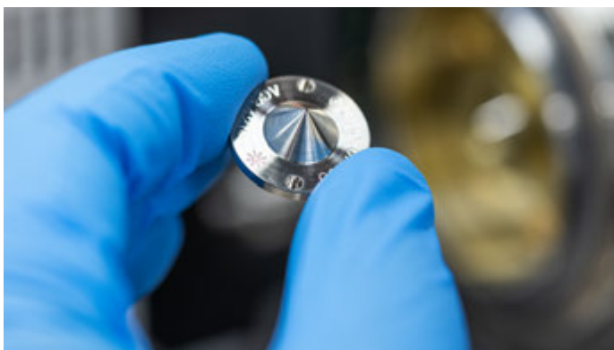
Figure 9. Brand new or thoroughly cleaned cones should be conditioned by running a moderate matrix prior to sample analysis. This creates an insulating coating that helps prevent drift.
