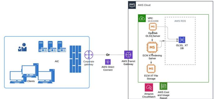
Example for AWS Hybrid Private Cloud Model configuration for OpenLab CDS
