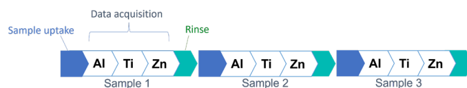
Figure 2. Sequential analysis of samples using multi-element sICP-MS method using the Rapid Multi-Element Nanoparticle Analysis module for Agilent ICP-MS MassHunter software.
