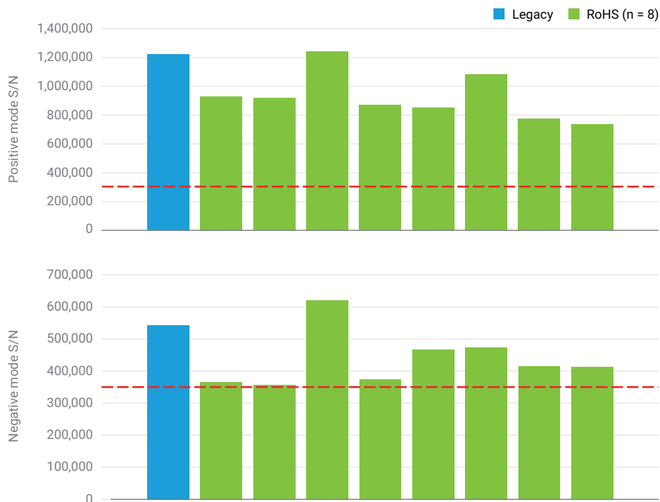
Figure 14. Comparison of S/N measurements on a 180 mm legacy Agilent FS ion injector versus a 180 mm RoHS Agilent FS ion injector (n = 8), in positive and negative mode, on an Agilent 6470B LC/TQ. A passing specification on the 6470B LC/TQ is 350,000:1 (marked by the red, dashed line).
