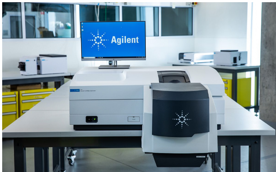
Figure 2. The Agilent Cary 7000 UV-Vis-NIR Universal Measurement Spectrophotometer.
