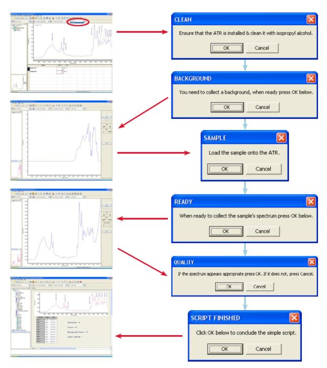
Figure 6. Automation of a standard operating procedure allows for high-quality spectra to be collected in seconds by novice users, reduces chances for protocol deviations and provides customizable printed reports that include advanced data interpretation
