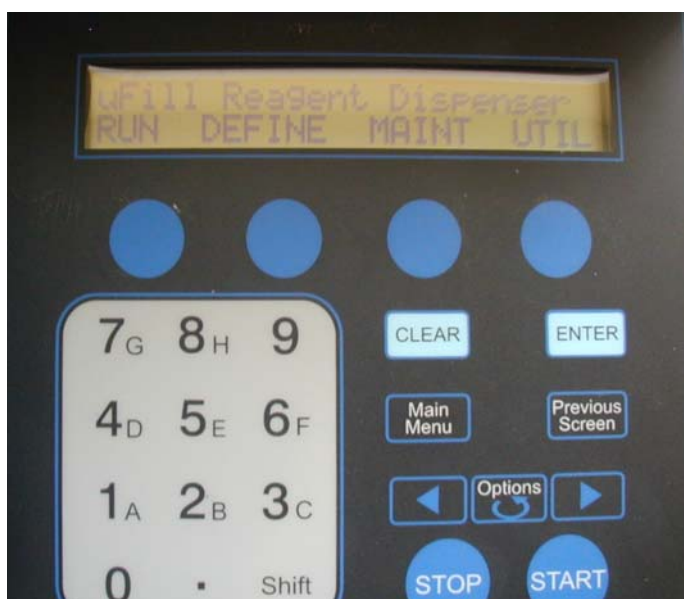
Figure 2. Programming Keypad for the \mu Fill Reagent Dispenser. Dispense programs, maintenance routines and instrument utilities can be accessed and programmed directly from the instrument keypad. Under the UTIL menu, select TESTS. To access the aspiration delay command, press the Shift and Hidden key #2 (area between the Main Menu and Previous Screen buttons) simultaneously. Select SYR then DELAY to define the length of aspiration delay in milliseconds.
