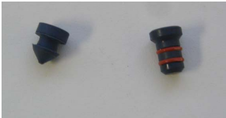
Figure 5. Original and New Manifold Plugs. The original style rubber manifold plugs (left) have been replaced with a more rigid design (right) that incorporates two O-rings to make a liquid tight seal.
