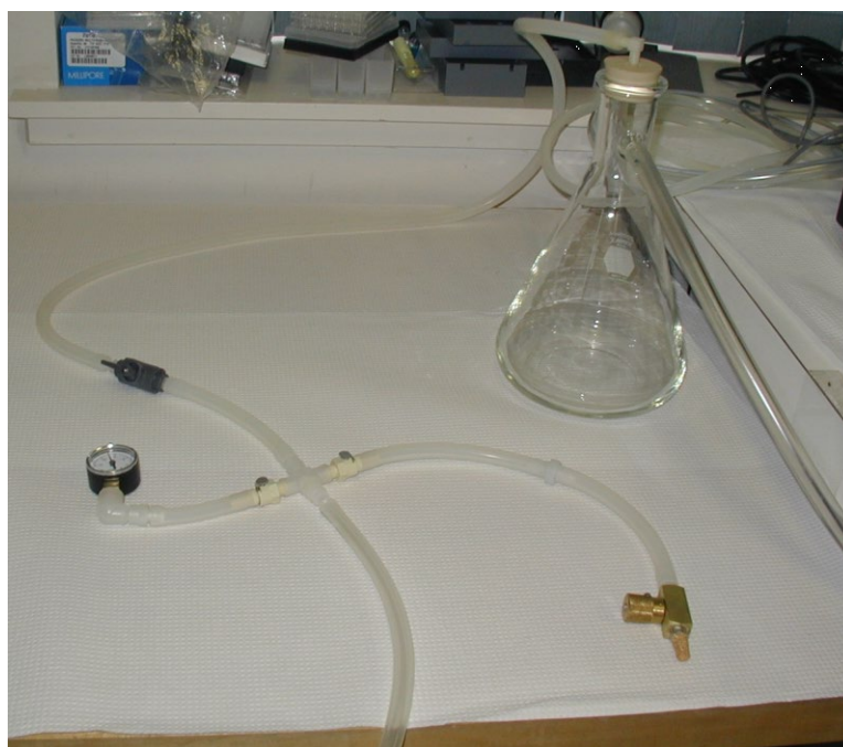
Figure 5. Tubing Connections of Millipore's vacuum apparatus. The pressure regulator, vacuum gauge, shutoff valve and pump are connected using 0.25" inner diameter tubing and quick-connect fittings.
