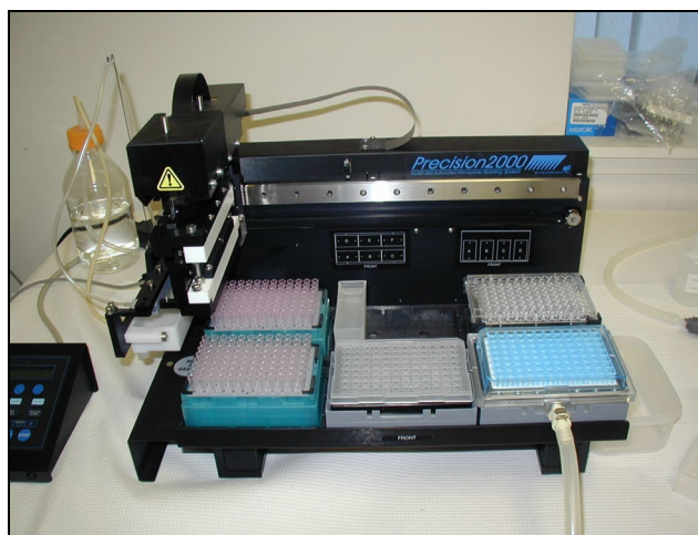
Figure 1. Precision™ Microplate Pipetting System with Populated Deck. The Precision™ Microplate Pipetting System has two boxes of pipette tips located in positions A and D. The Montage™ SEQ 96 plate and vacuum manifold has been located at position C using a holder (P/N 7112110) designed to accommodate the tubing connector in the front. A separate holder (P/N 6002076) is used to secure a 96-well skirtless PCR plate and then positioned on the deck at position B using the same holder as the vacuum manifold. Injection solution is located in the reagent reservoir at position E, while the injection plate is located at position F.
