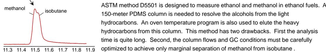
ASTM method D5501 is designed to measure ethanol and methanol in ethanol fuels. A 150-meter PDMS column is needed to resolve the alcohols from the light hydrocarbons. An oven temperature program is also used to elute the heavy hydrocarbons from this column. This method has two drawbacks. First the analysis time is quite long. Second, the column flows and GC conditions must be carefully optimized to achieve only marginal separation of methanol from isobutane.
