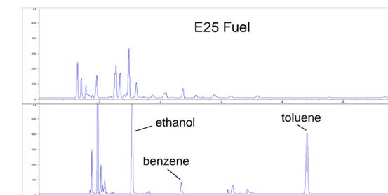
Commercial ethanol fuels are made by blending denatured fuel ethanol with various ratios of petroleum gasoline. The ethanol, methanol, benzene and toluene content must also be measured in these fuels. Two samples of commercial ethanol fuels, E25 and E85, were obtained and run along with the denatured fuel ethanol using this MDGC method. Three consecutive runs were made for each sample. The table below shows excellent precision for each sample
