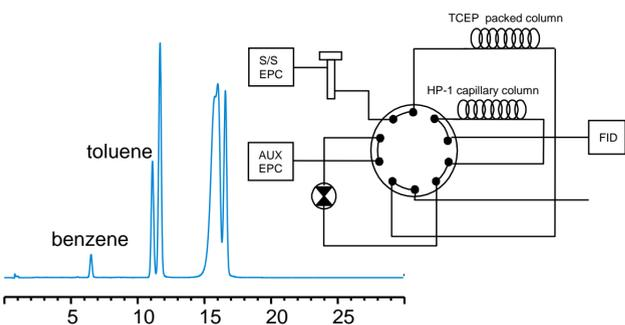
ASTM method D5580 is specified for the measurement of benzene in ethanol fuels. This method uses a 12-port valve and a two columns to separate benzene from the ethanol and hydrocarbons in the sample. While this method works quite well, it does require a lab to have another GC to completely measure key components in ethanol fuels.
