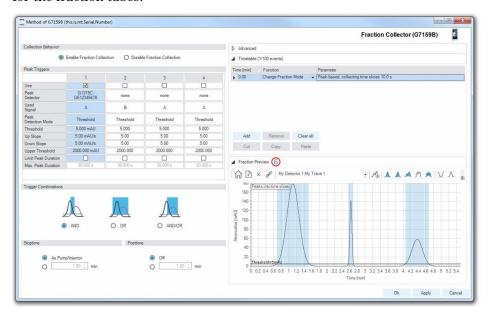
**6** The Fraction Preview is now accessible from within the method user interface. This function is especially useful when the user wants to do multiple injections of the same compound without changing any parameter.
