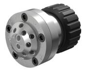
The G4734A 6-Position/14-Port Valve is designed to allow switching between up to 6 preparative columns. This versatile valve is rated for a maximum flow rate of up to 200 mL/min and can withstand a maximum pressure of 600 bar. The G4734A can also be used as clustering valve for Fraction Collectors.
