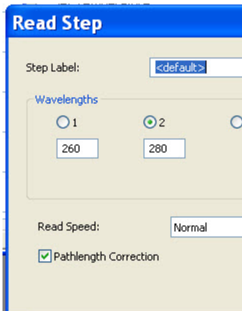
Figure 10: During sample measurements path length correction is selected for determination of the variable path lengths inherent with microplate measurements.
