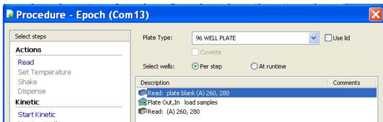
Figure 9: During microplate analysis of dsDNA samples the plate is first pre-read for blanking followed by sample loading and measurements at 260 and 280 nm using a standards Gen5 protocol.
