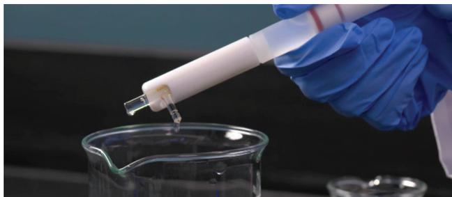
Backflush with a suitable cleanser, such as methanol or a 2.5% detergent solution. We recommend using a dedicated [nebulizer cleaning tool](#) (p/n G3266-80020).
