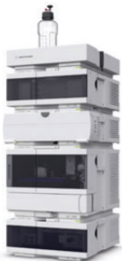
Figure 1. The optimized system for GPC. An Agilent 1260 Infinity II GPC/SEC system.
