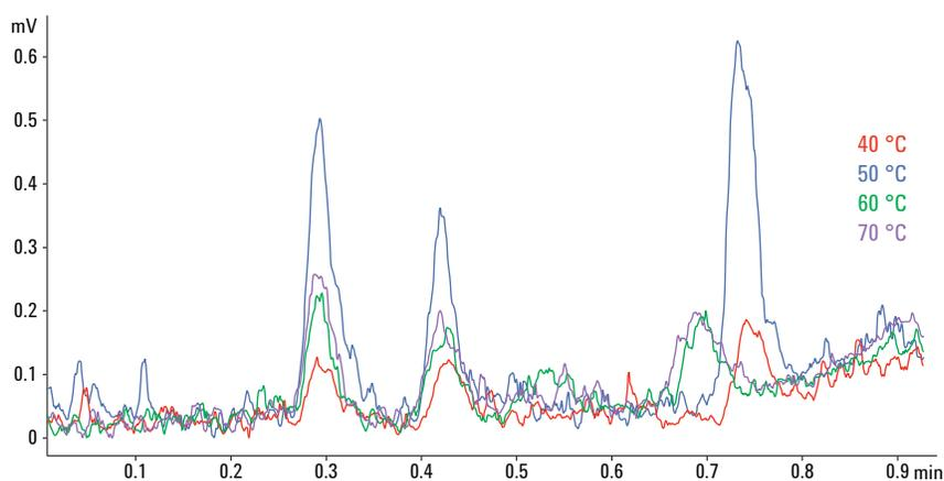
Figure 5. Overlay chromatograms of amino acids (0.1 mM) with different evaporator temperatures.
