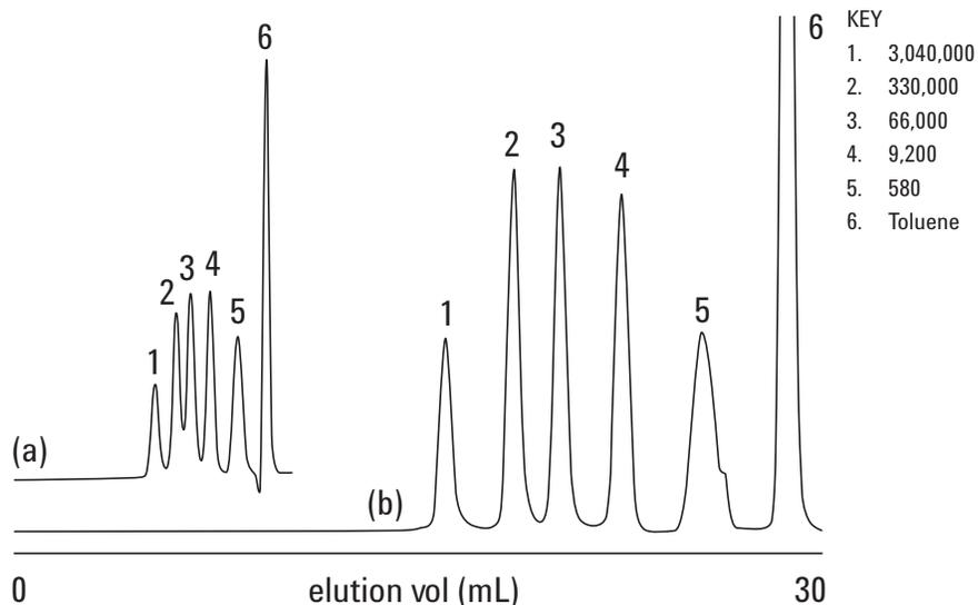
Figure 1. Effect of column length on separation. a) single Agilent PLgel 10  $\mu$ m MIXED-B columns, b) three PLgel 10  $\mu$ m MIXED-B columns.
