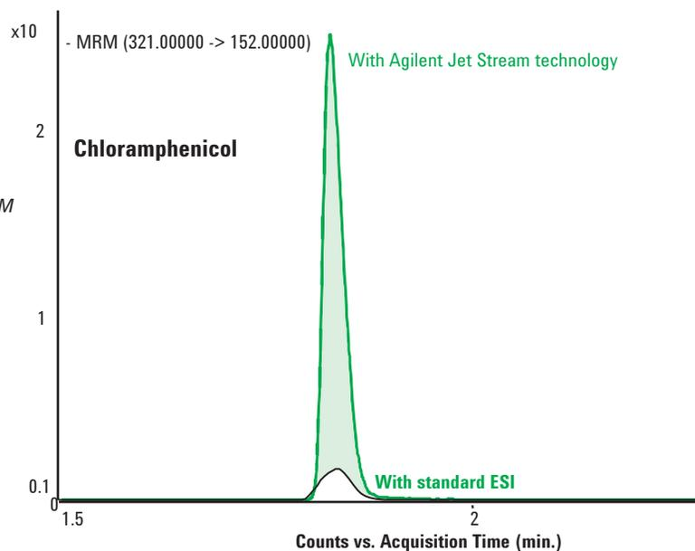
Figure 2. Comparison of the MRM intensity for chloramphenicol spiked into potable water analyzed in negative ion mode. Injected volume was 5  $\mu$ L of a 50 ppb solution.
