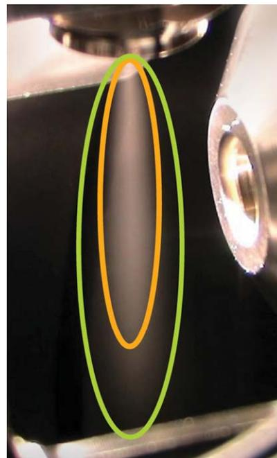
Figure 1. Agilent Jet Stream Spray Confinement
