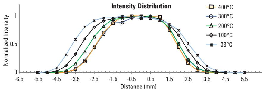
Figure 3. Normalized ion intensities as the spray plume from AJS is moved laterally off-center. The highest ion intensity occurs in a 3-5 mm wide band in front of the sampling capillary.
