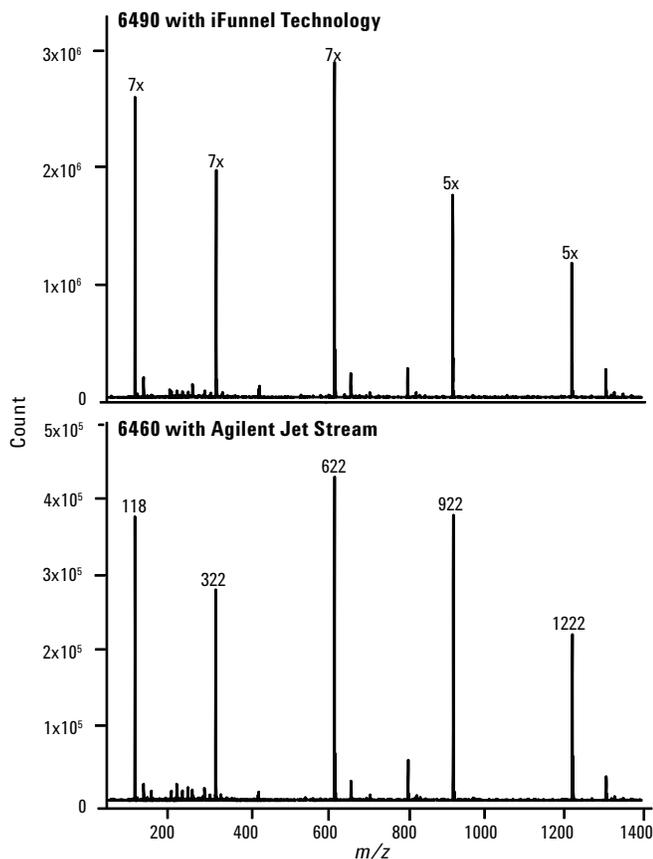
Figure 7. Signal intensities for calibration standards in positive ESI for 6490 Triple Quad (top) and 6460 Triple Quad (bottom) show increases across a wide mass range.
