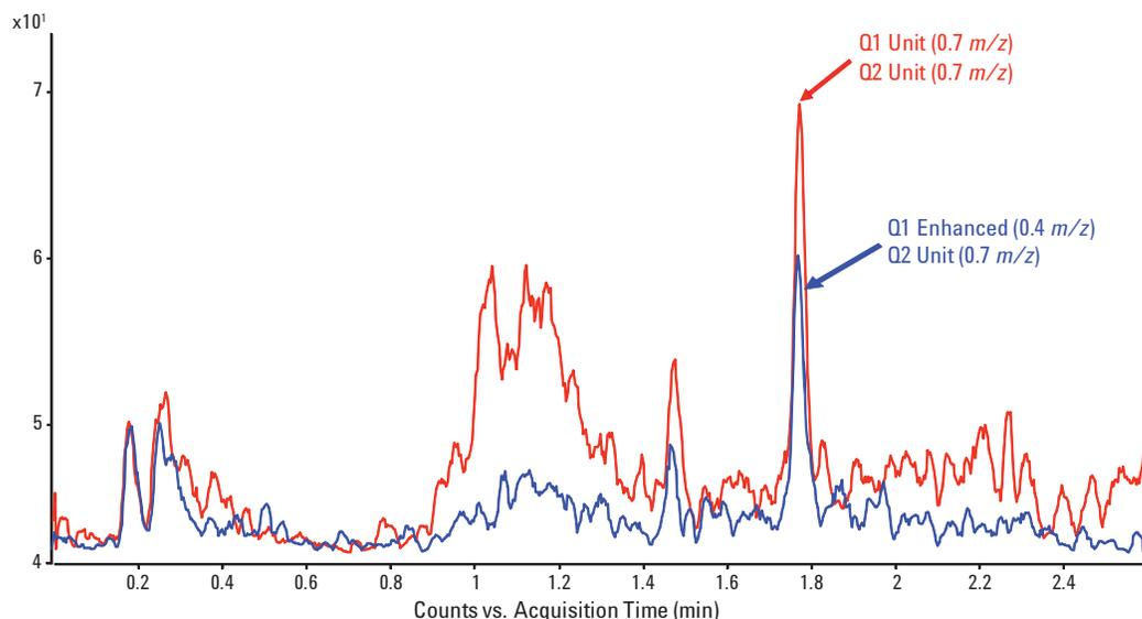
Figure 10. 2.5 fg of fluticasone propionate from a plasma sample. MRM data using a precursor isolation resolution of  $0.7\ m/z$  (red) and  $0.4\ m/z$  (blue). Narrow isolation reduces non-specific signal and improves detection limits.
