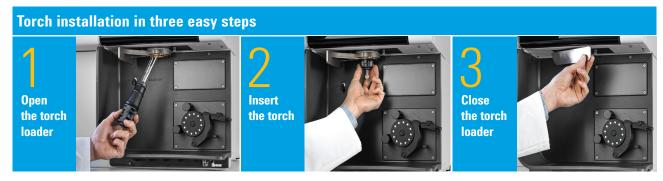
Figure 2. Sequence of 3-easy steps to load the torch into the instrument for fast start up and reproducible performance.
