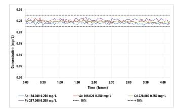
Figure 3. Stability test over 4 hours for a 0.25 mg/L multi-element spike in 25% NaCl.
