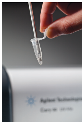
Figure 4b. Measuring down to 140 \mu\text{L} in 0.5 mL microcentrifuge tubes using the fiber optic micro probe and the Cary 60.
