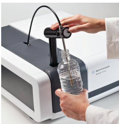
Figure 4a. Measuring samples with the standard fiber optic probe and the Cary 60. Take the instrument to the sample.
