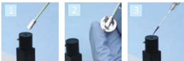
Figure 1. The ultra-microvolume cuvette for the Cary 60 is easy-to-use and easy to clean. Simply drop a sample onto the platform, replace the reflective lid, and take a measurement.
