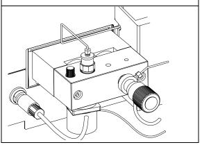
3 Clean the pump chambers, ensure all particulate matter is removed. Best cleaning results will be achieved by removing all three valves (see pages 103, 106 and 108) and injecting solvent into each chamber.
