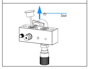
1 Disassemble the pump head assembly (see "Removing and Disassembling the Pump Head Assembly" on page 110).
