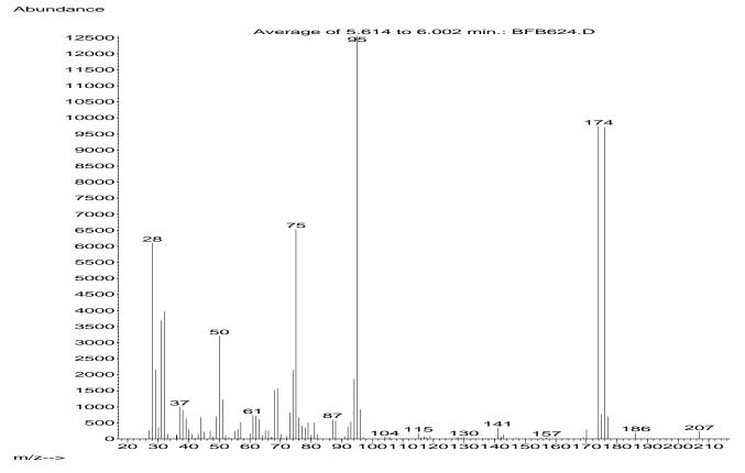
Notice a y-axis abundance for mass 95 of 12,500 counts. If this same solution is used over time, the abundance of mass 95 may be getting smaller. This in turn will usually make the ratio of the 174 also to go down, resulting in the failure to pass the EPA criteria at the higher mass fragment. This is normally due the evaporation of the BFB, which in turn makes the concentration of the BFB lower than what was originally prepared.
