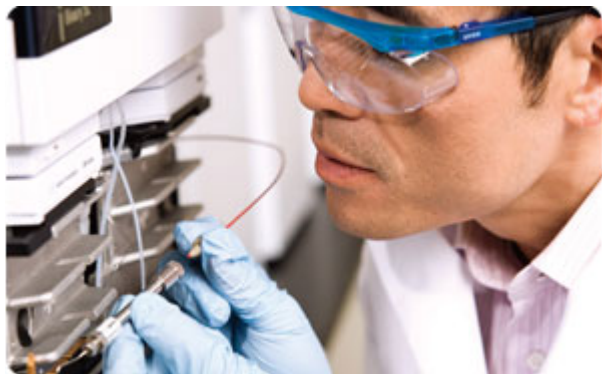
Figure 3. To avoid contaminating the flow cell while cleaning the column, disconnect the column from the detector and divert the effluent flow directly to a waste container.
