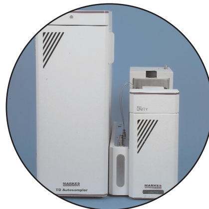
UNITY 2 configured for both tube and canister/on-line automation
